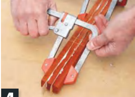
4 Cramp the three lengths together, with veneer strips sandwiched in between. Adjust, as the timber will slide when tightening cramps
